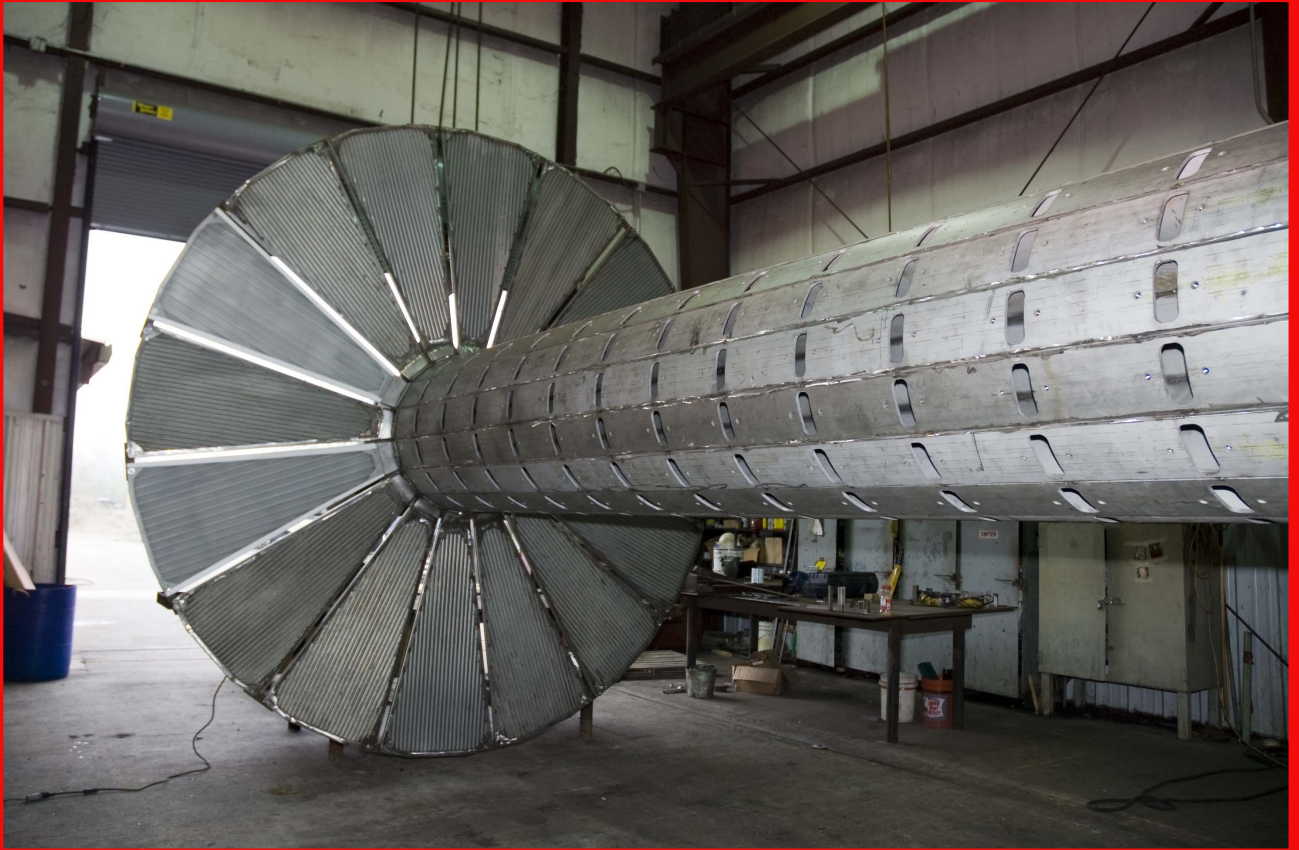
Compositech Centerbarrel for Disc filter in process (pictured) built for Georgia Pacific
