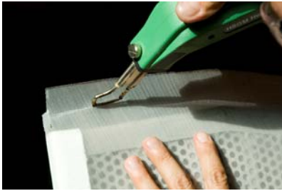
Sector Cover Cut To Size With Heat Knife
