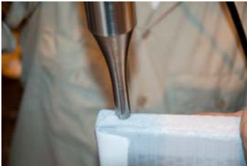
Ultrasonic Welding of Sector Cover
